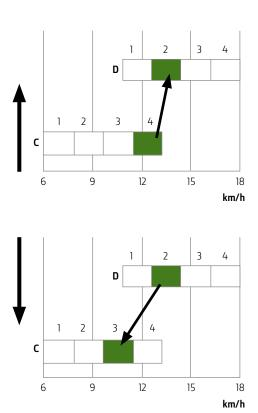
Speedmatch ensures that when you're shifting range with a Powr8<sup>™</sup> or PowerQuad<sup>™</sup>, the transmission always selects the best gear to match the tractor's forward speed.
